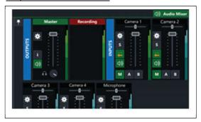
Audio Mixer allows you to easily keep track of all audio sources and includes the ability to Mute, Follow (Auto Mixing) and Delay any source.
