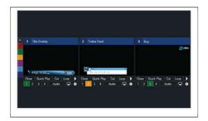
StudioCast includes 4 Overlay Channels in addition to the Multi View feature. Each overlay channel can have its own transition effect, position and border.
